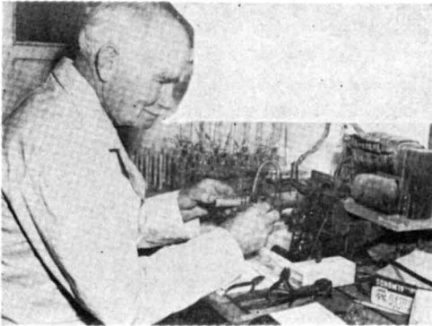
Dr. Lee De Forest making radio tubes with an Eisler spot welder.
